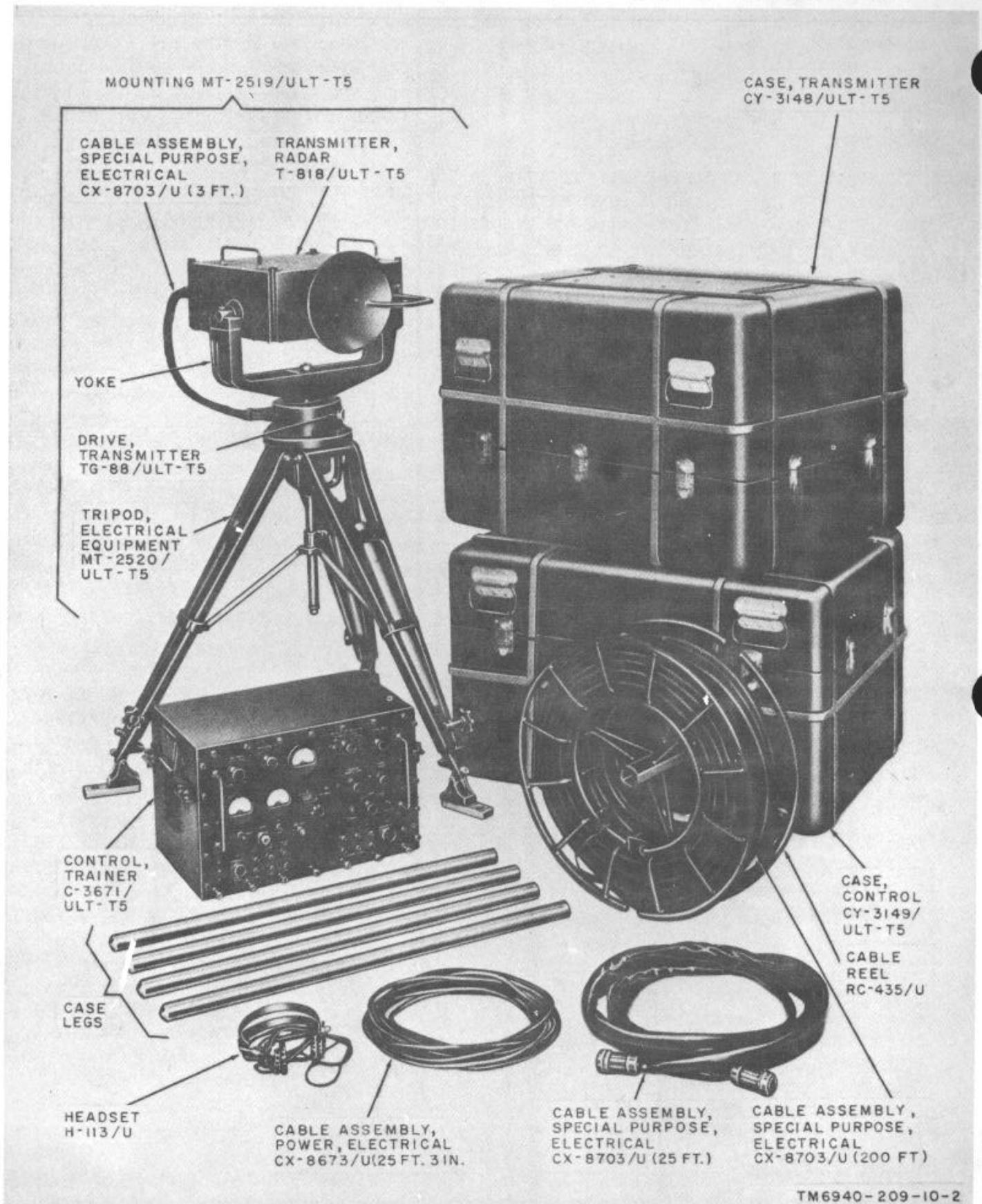
Figure 2. Radar Trainer AN/ULT-T5, components.
